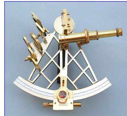
Sextant—used for determining latitude—replaced astrolabe b/c more precise
