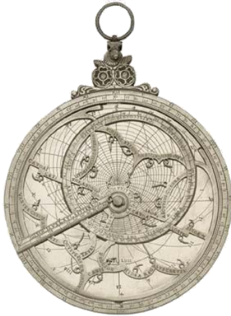
Astrolabe, used to measure latitude
